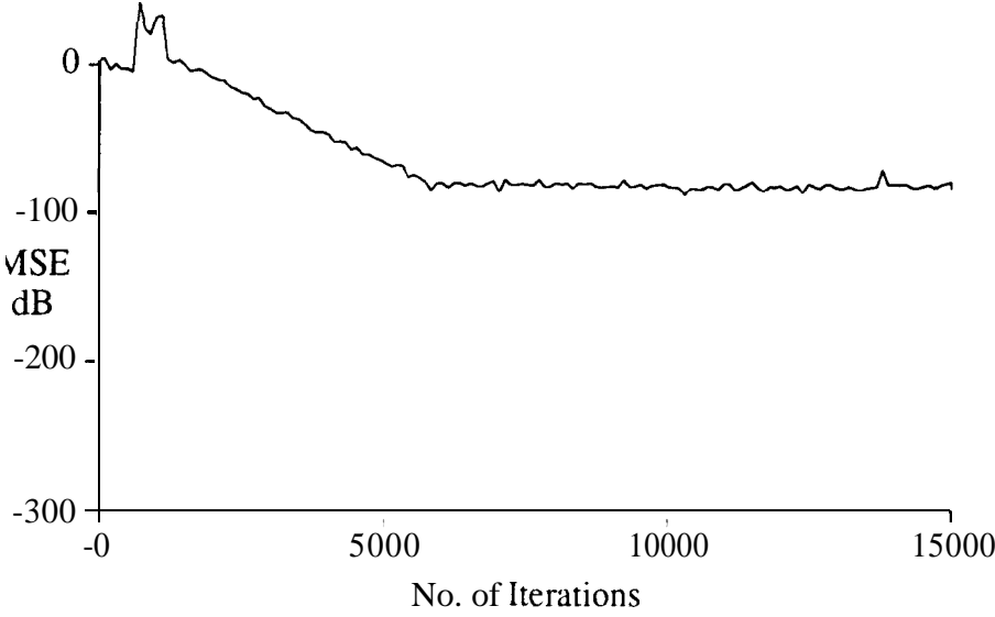
Fig.3.10 Convergence curve for BCF with measurement noise of 26 dB. Step size for all-pole second-order sections = 0.004 and step size for transversal section = 0.049.
