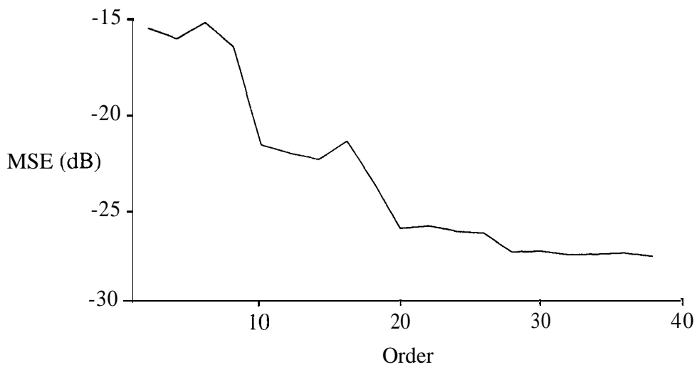
Fig.6.14 MSE versus order of an adaptive backpropagation filter.
