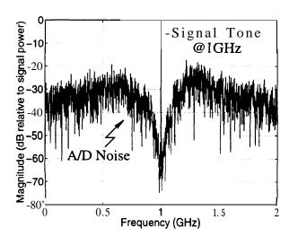
Fig. 8. Simulated output spectrum of a fourth-order LC bandpass modulator.
