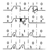
Fig. 1. Illustration of NRZ nonlinearity. (a) NRZ ( $0\ 1\ 0\ 10$ ) pattern. (b)NRZ ( $0\ 1\ 10$  0) pattern.(c) RZ( $0\ 1\ 0\ 1$ ) (d)RZ( $0\ 1\ 1\ 0\ 0$ ) pattern.
