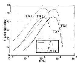
Fig. 2. Measured  $f_t$  and  $f_{\rm max}$  versus  $I_C$  for both TX1 and TX6 transistors at  $V_{CE}=1\,$  V.
