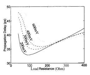
Fig. 4. Propagation delay versus load resistance for the latching comparator with different differential voltage swings.
