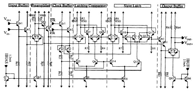
Fig 3. A complete schematic of the SiGe HBT return-to-zero comparator
