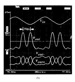
Fig. 6. Simulated and measured waveforms for the SiGe HBT comparator with sinusoidal inputs: (a) simulation and (b) measurement.
