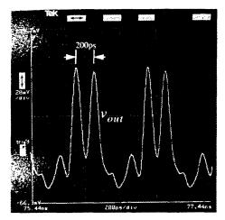
Fig. 7. A measured output waveform in response to a I.25 GHz input signal and a 5  $\,GHz\,$  clock.
