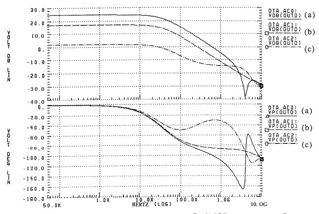
Fig. 6. OTA frequency response for a setting of (a) maximum  $G_m$ , (b)  $0.5G_m$ , (c) a low value for  $G_m$ .
