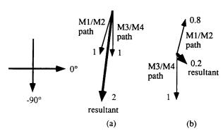
Fig. 5. Illustrating magnitude and phase of output signal for two possible  $G_m$  settings. (a) maximum  $G_m$ ; (b)  $0.2G_{m,\max}$ .
