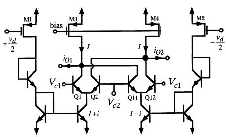
Fig. 2. The basic transconductor illustrating tuning mechanism.
