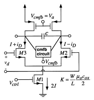
Fig. 1. A simple tunable transconductor integrator,
