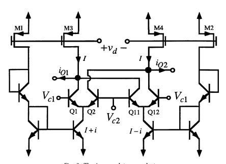
Fig. 3. The improved transconductor.
