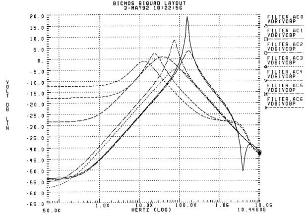
Fig. 10. Bandpass function frequency response for various  $f_o$  and Q settings.
