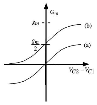
Fig. 4. Transconductance characteristics a, b for the transconductors in Figs. 2 and 3, respectively.
