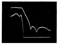
Fig. 6. Measured response of the fifth-order elliptic single op-amp  $\Delta$  domain low-pass filter.horizontal 0.2 kHz/div. Vertical: 10 dB/div. (upper trace), 1 dB/div. (lower trace).
