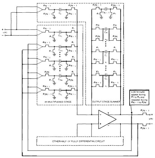
Fig. 2. Generalized multiplexed SC realization for  $\Delta$  domain state-space structures
