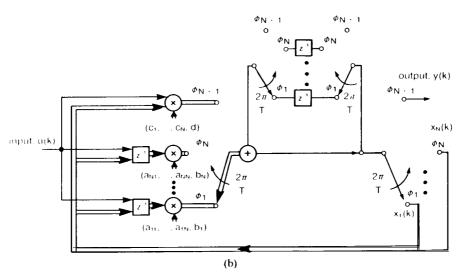
Fig. 1. Functional representation of A domain state-space Structure in (a) nonmultiplexed form and (b) multiplexed form.
